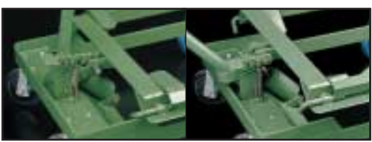
the shock absorber ensures the storage containers are set down slowly
