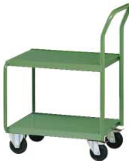
Art. F CR 0031 00 02 green Art. F CR 0031 00 04 blue Stacking and storage container trolley 2 swivel wheels in rubber Ø 125 mm with brake 2 fixed wheels in rubber Ø 125 mm Overall dimensions: mm 765x560x1030h Load kg 250
